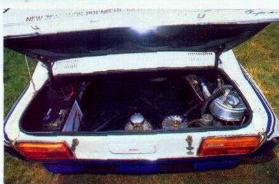
Bottom, note the dry sump oil tank and boot and huge intakes for the side-mounted water radiators
